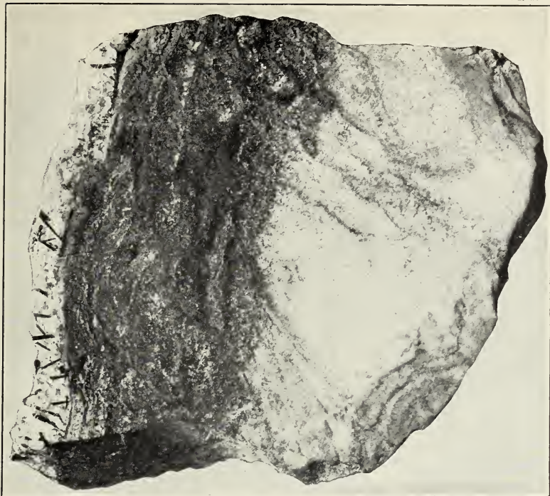
A. POLISHED SURFACE OF WALL ROCK ADJOINING WOLFRAMITE-QUARTZ VEIN. Showing marked contrast between the marmorized limestone and the metasomatically altered limestone.
